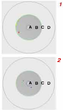
Image 1: Three (3) defects in the cladding zone. Those highlighted in red are over 5 \mu\text{m} in diameter causing a failure condition.
